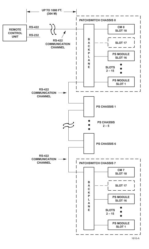
Figure 2-4. RCU to Local PatchSwtich Chassis, Interconnection Block Diagram
